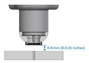
To successfully execute the Screwdriver commands, it is fundamental to operate the Screwdriver downwards or maximum sidewards. The Screwdriver should not be operated upwards or with an angle higher than 90° orientate with respect to the ground, since this will trigger the protective feature.
