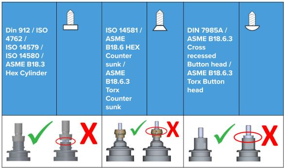
4. When this is achieved, remove the screw and push in the screw fix (only Din 912, ISO 4762, ISO 14579, ISO 14580 and ASME B18.3 HEX Cylinder screw types).
