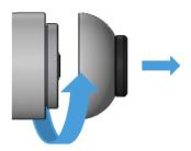
Place the hex shape of the bit holder inside of the end of the Screwdriver's shank. The system will be attached to the Screwdriver by a magnetic force.
