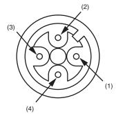
Applicable connector code: XS5F / XS5W series Applicable IO-Link master unit: NX/GX series
