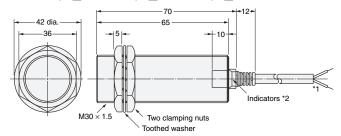
\*1. 6-dia. vinyl-insulated round cable with 2 conductors (Conductor cross section: 0.5 mm2, Insulator diameter: 1.9 mm), Standard length: 2 m 6-dia. vinyl-insulated round cable with 3 conductors
