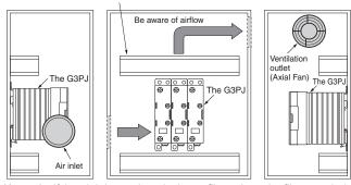
Note: 1. If the air inlet or air outlet has a filter, clean the filter regularly to prevent it from clogging to ensure an efficient flow of air.
